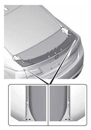
20. While applying light pressure on the trunk spoiler, carefully remove the adhesive backings.
