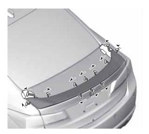
21. Firmly press the trunk spoiler against the trunk lid. Remove templates C.
