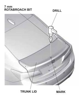
10. While wearing eye protection, use a 8.5 mm Rotabroach bit to drill the trunk lid at the outer centerpunched marks.
