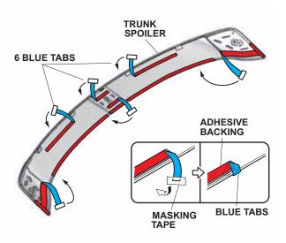
16. Partially peel back the 5 adhesive backings, and tape them to the front of the trunk spoiler with masking tape. Leave as much of the adhesive covered as possible.
