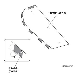
6. Place template B on the trunk lid, insert the six tabs and align it with the left edge of the trunk lid. Tape template B to the trunk lid with two pieces of masking tape.
