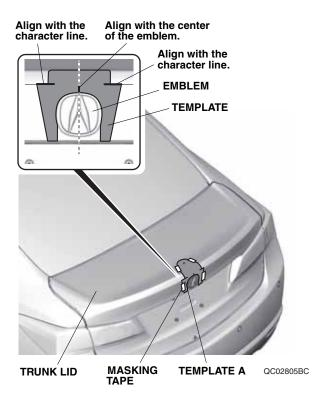
4. Set a center punch to the minimum power setting, and mark the trunk lid through the hole in template A. Remove template A.
