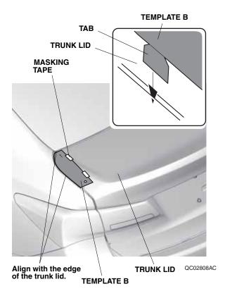
7. Using the center punch, mark the trunk lid through the hole in template B. Remove template B.
