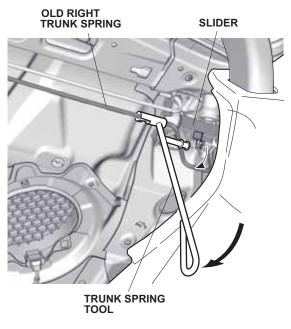
Remove the spring from the hinge bracket.
