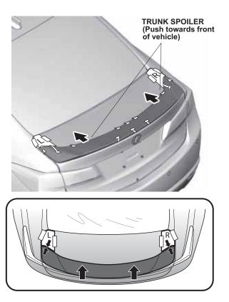
19. Adjust the position of the trunk spoiler so there is equal spacing on both sides.
