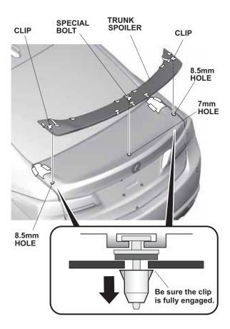
18. Push the trunk spoiler towards the front of the vehicle as shown, and align the spoiler with the left and right templates.
